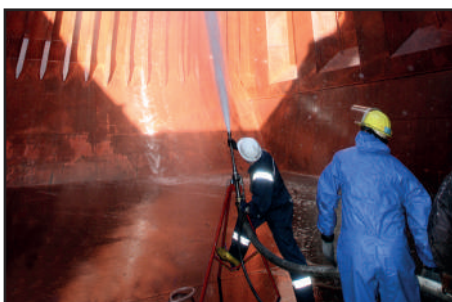
HOLD TANK CLEANING
